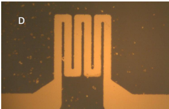
Fig 11 (A) , (B), (C), (D) shows resistive patterns of varying dimensions and the resistances offered.
