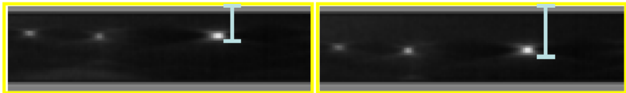
Figure 5. The left picture shows the depth of a fluorescent bead in a collagen hydrogel. The right image then shows the new depth of that same bead during the portion of the ultrasonic therapy cycle when the acoustic force is applied (unpublished data).
