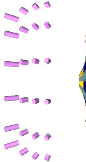
FIG. 17: A side view of the HTCC mirrors and PMTs.
