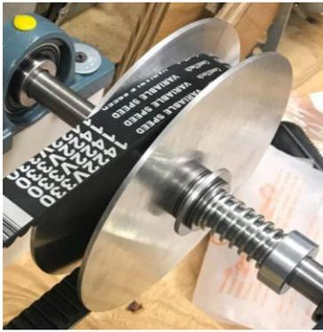
*Figure 3, Close-up of actuation method*
