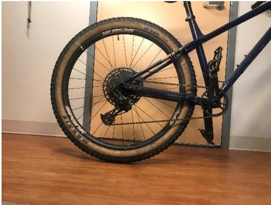
*Figure 1, Derailleur based drivetrain*
