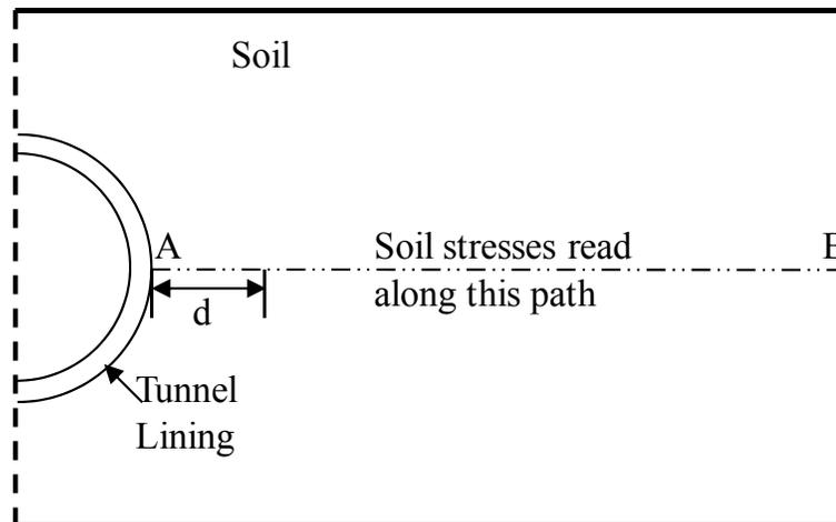
Figure 8. Path AB along which stresses in soil are studied
